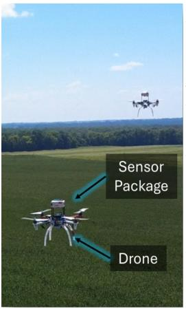
deploying swarms of drones to track airborne pollutants emitted from swine barns. Their research focuses on how contaminants like particulate matter (PM), ammonia (NH $\square$ ), and hydrogen sulfide (H $\square$ S) disperse into surrounding communities—potentially affecting air quality and public health.
