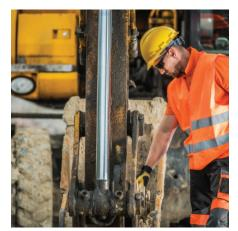
If a quick coupler or an attachment needs to be inspected, do not approach the device unless the attachment is lowered and resting on the ground. This is equally important for manually
